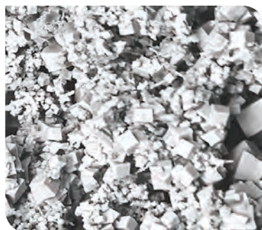
Microscopic view (x5000) of well developed copper hydroxide \{Cu(OH)_2\} protective layer formed on the inner surface of TALOS® copper tube.
