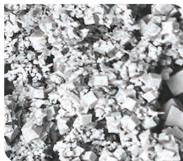
Microscopic view (x5000) of well developed copper hydroxide {Cu(OH) 2 } protective layer formed on the inner surface of TALOS® copper tube.
